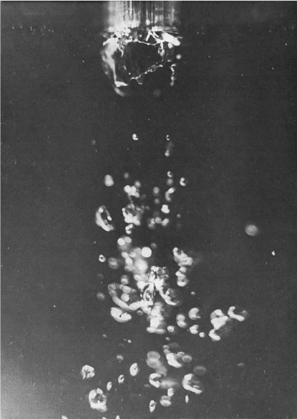
FIGURE 1. Water jet falling into a pool of water at rest. The camera looks at the free surface slightly from below. A short film of air envelops the jet around its entry point into the receiving liquid, clearly visible at the top of the figure. The diameter of the jet is slightly less than 1 cm and its velocity about 0.7 m/s. (Courtesy of Professor J. Duncan.)
